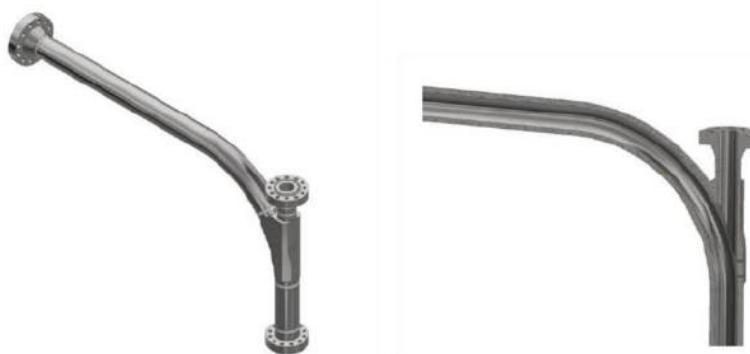
Figure 16: Vertical access in spool for allowing the insertion of hydrate removal equipment into subsea lines
